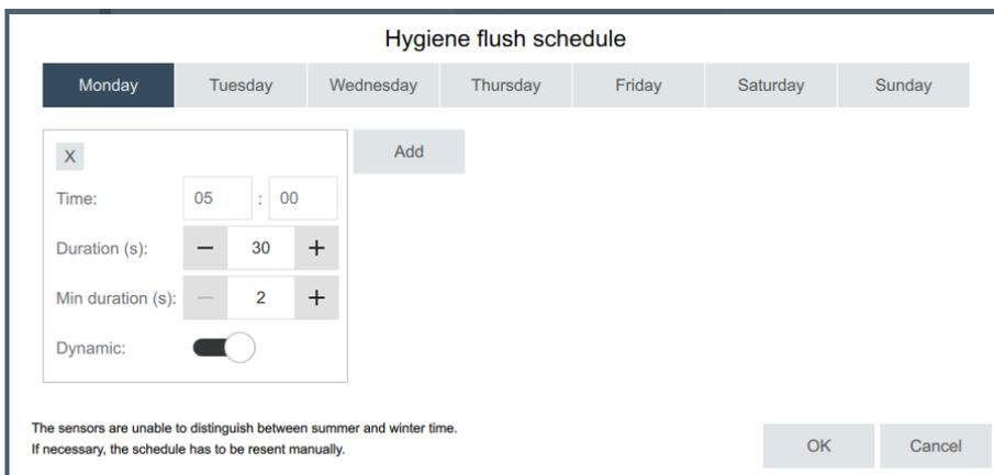
6. Specify the time when the flushing should take place as well as **"duration"** and **"min duration"**.
